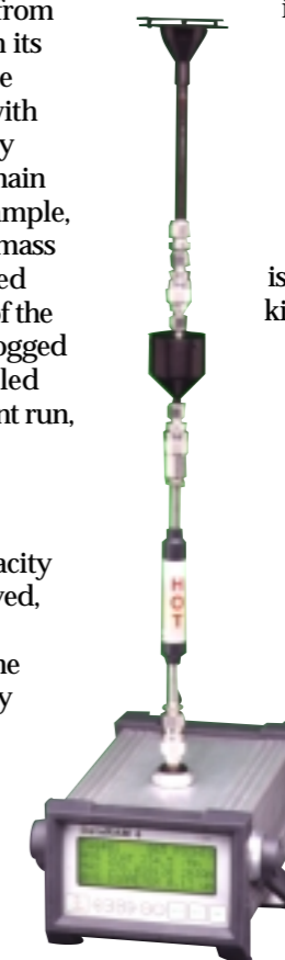
DataRAM 4 with ambient monitoring accessories
