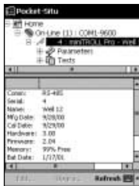
Select the device to display its information including remaining battery and memory.
