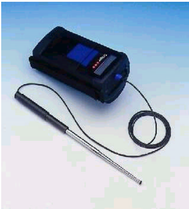
CMS System with Remote System and Probe
